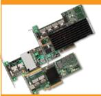
The MegaRAID SATA+SAS value line offers a mix of value and performance for internal SATA and SAS systems. These products feature 3Gb/s or 6Gb/s transfer rates, internal connectivity and support for both SATA and SAS drives.
